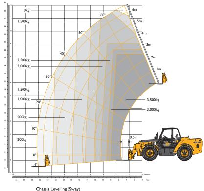
With stabilisers retracted (Sway angle  $\pm 9^{\circ}$ )
