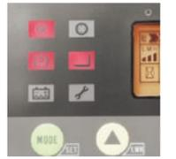
The interlock state is also indicated on the meter panel.
